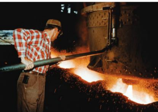
▲ Worker opens the nozzle of a ladle to pour molten steel into ingot moulds in Volta Redonda, Brazil, 1995
